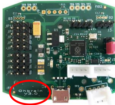
Ohbrain V3.0 (Headroll motor connects to pins JP10)
